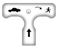
There is a glow-in-the-dark trunk release handle located on the latch inside the trunk . This handle will glow following exposure to light. Pull the release handle to open the trunk from the inside.
